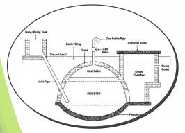
Capable of handling 50 Kg to 1 Ton of biodegradable waste per day. It is constructed using ferro cement.
